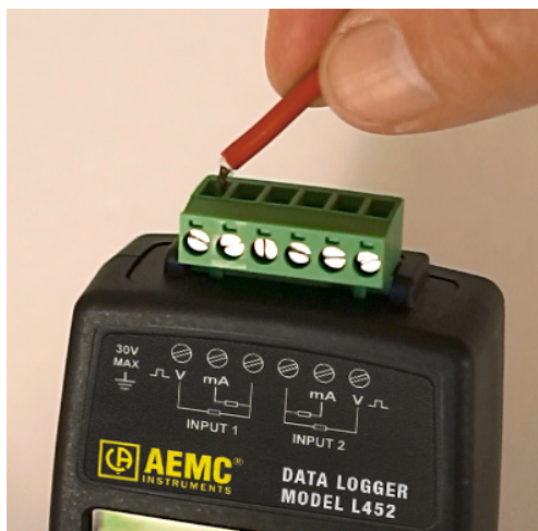
Figure 24. Inserting a lead into the terminal strip
